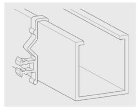
Open the gate of the box brackets and slide the headrail into position then snap the brackets closed.
