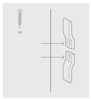
Wrap the cords around the cord cleats in a figure of 8. When the cords are fully accumulated ensure they are secure so when any cord is pulled no excess cord is released.
