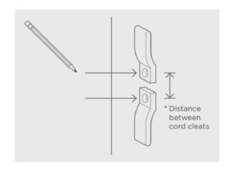
Use the screws provided to attach the safety cleat to the wall.
