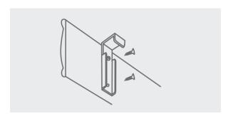
Hook valance clip with valance attached onto the top of the headrail.
