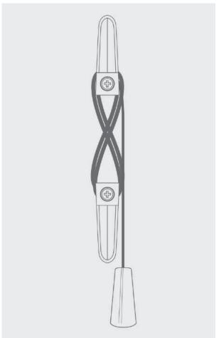
**To tilt blind:** Pull on required tilt cord tassel to tilt slats to the open/closed position.
